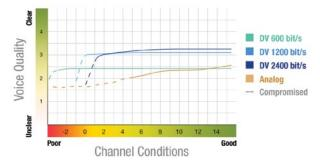
When analog SSB mode is needed, Envoy's patented *Easitalk*<sup>™</sup> DSP algorithm works to actively remove background noise and interfering ones. During transmission, Codan's TalkPower feature dynamically compresses and shapes the frequency response of the voice signal to maximise transmit power and intelligibility. A syllabic squelch only opens the speaker mute when speech signals are present to eliminate background noise.
